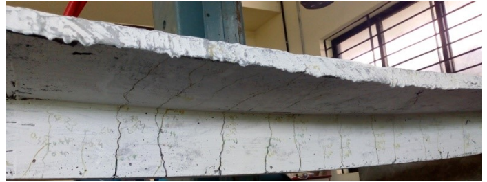
Fig 7: Crack pattern in HC T-beam
