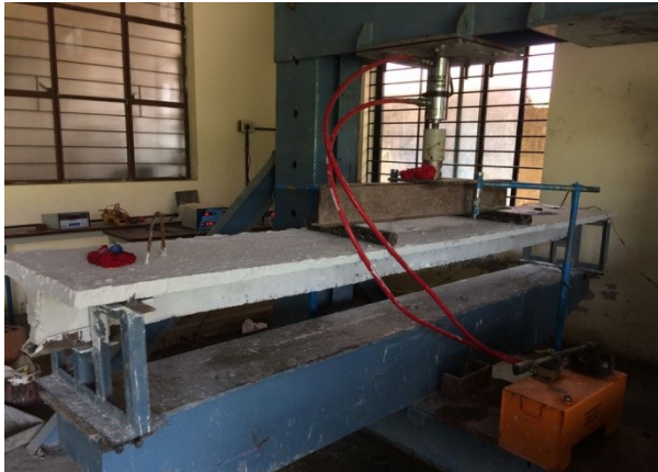
Fig 4. Test setup for T-beam
