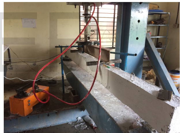
Fig 3. Test setup for rectangular beam
